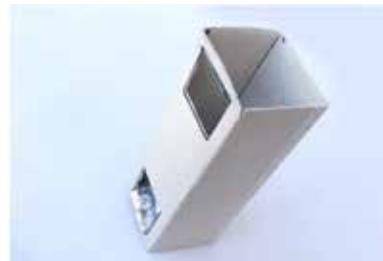
The mirrors should be positioned at 45 degrees to each other and your periscope is now ready for action.
