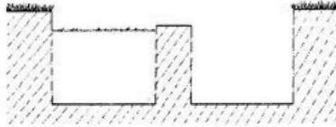
Combined dry and wet waste pits built to take off the turf in one piece, showing grease trap.
