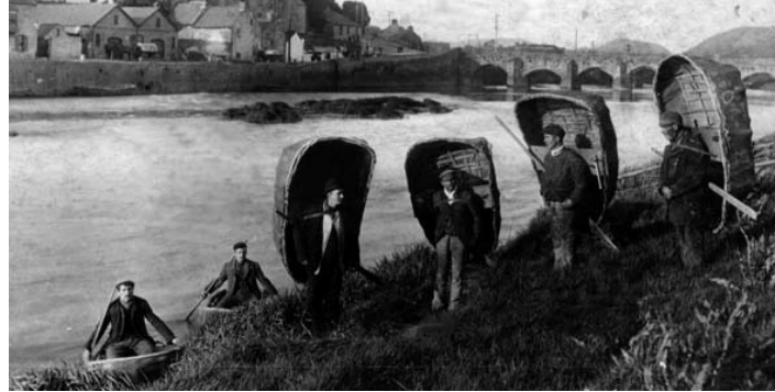
The picture shows traditional Welsh coracle circa.1890. This craft is built using ash lathes and covered with cowhide.
