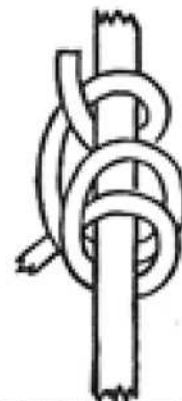
ROLLING HITCH is used instead of clove, and for guy lines.
