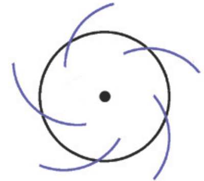
The barrel is divided into five panels - you will need a protractor to get the right spacing of the panels - 360 degrees dived by 5 = 72 degrees.
