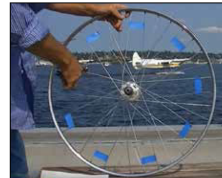
Mark with tape the spokes you wish to keep and remove other spokes.
