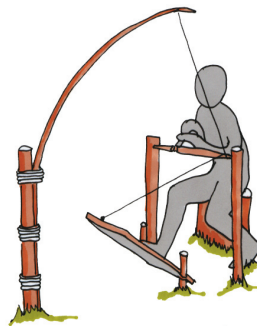
Traditional bodgers lathe using pedal power to turn a spindle. A grinding machine and multi purpose lathe make from the frame of an old bike
