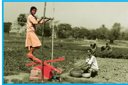
Simple Treadle pump in use in India
