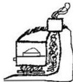
Traditional clay oven - barrel bridges fire pit, chimney constructed of tin cans
