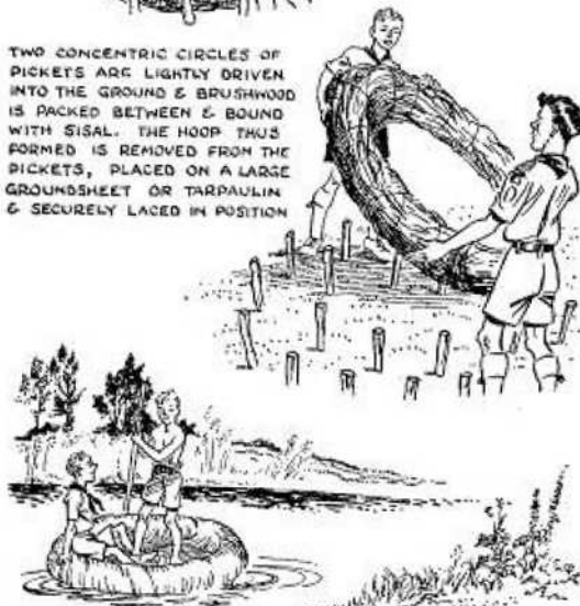
Coracle built from sticks and a groundsheet.
