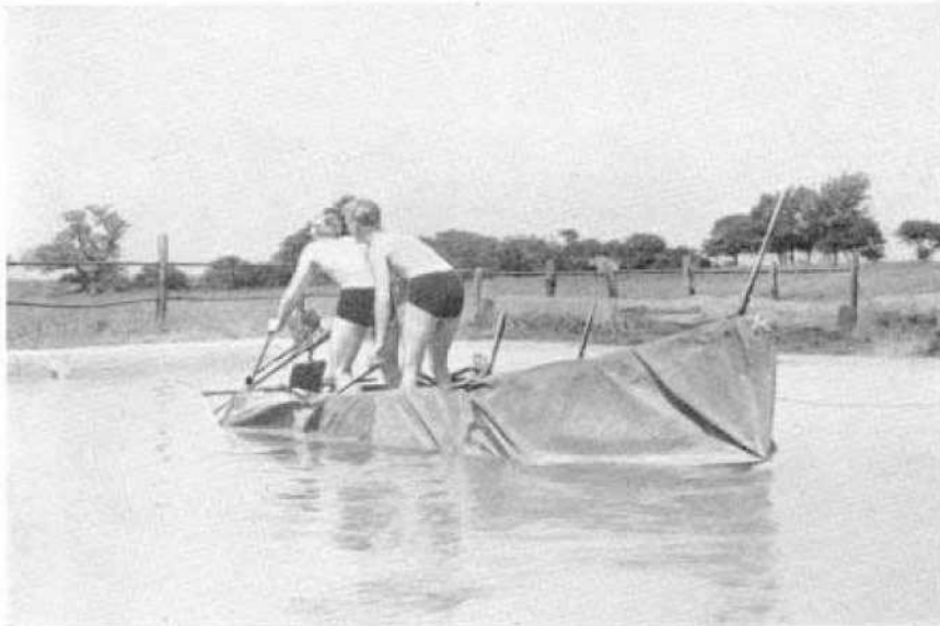
TARPAULIN RAFT WITH OUTBOARD MOTOR
