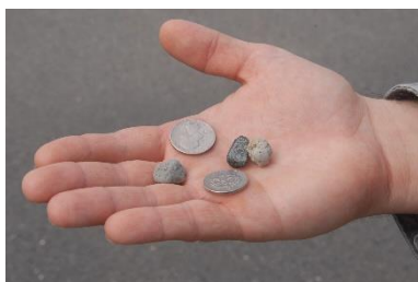
FOD collected at an Airfield
