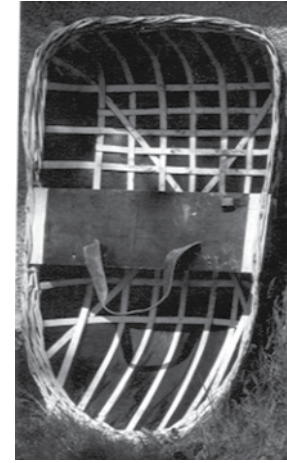
The picture shows traditional Welsh coracle circa 1890. This craft is built using ash lathes and covered with cowhide.
